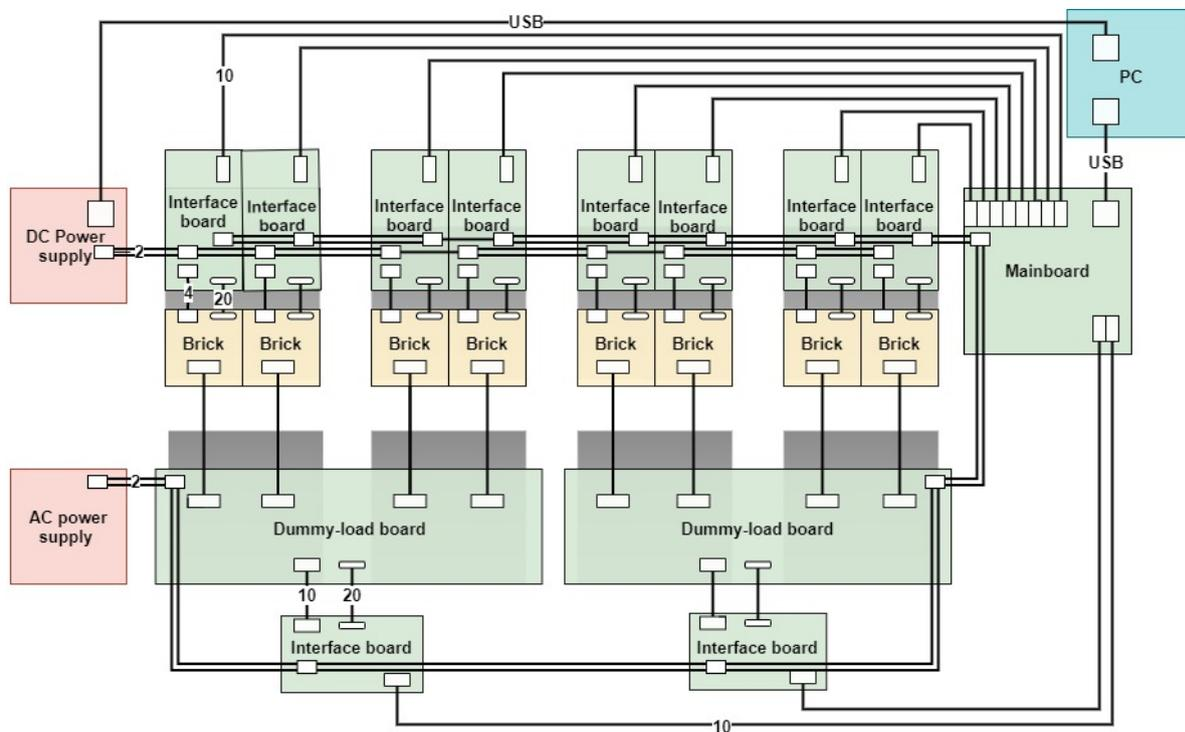
**Figure 2.** A block diagram of the Burn-in station hardware.
